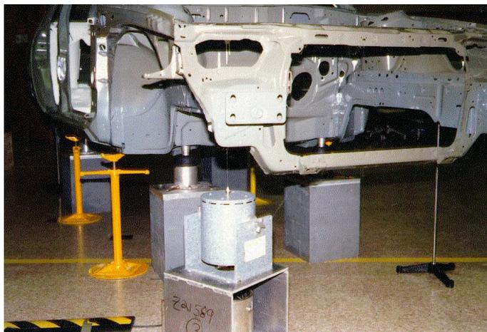
The MODAL 50A (and multiples thereof) is ideal for exciting structures smaller than say, a full-size automobile. Total vehicle modal tests on anything larger (truck, jet, even a space shuttle) requires multiple MODAL 50A's or the MODAL 250A.
