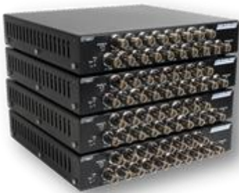
64 channel USB-frontend for Sound & Vibration 24-bit A/D, IEPE supply, RPM input, dig I/O
