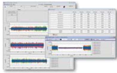
Drive-File development - Cut & Paste from different test tracks, PSD calculation & level statistics
